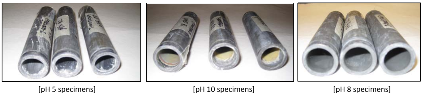
Figure 4: Pipe sections after exposure
