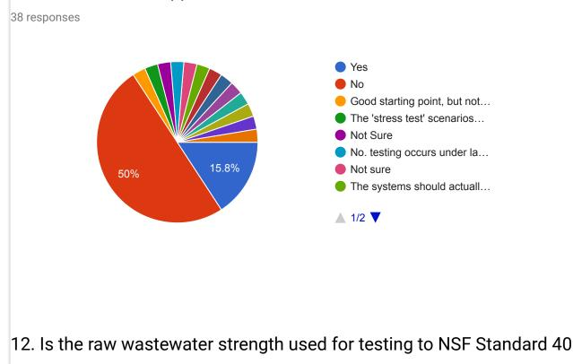
representative of typical residential sewage?From NSF/ANSI 40:The 30 d average BOD5 concentration of the wastewater delivered to the system shall be between 100 mg/L and 300 mg/L.The 30 d average TSS concentration of the wastewater delivered to the system shall be between 100 mg/L and 350 mg/L.
